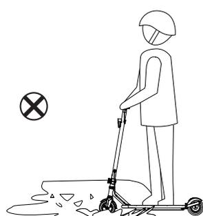
10. Do not immerse the product in water to avoid damage to the electrical parts of the vehicle.
