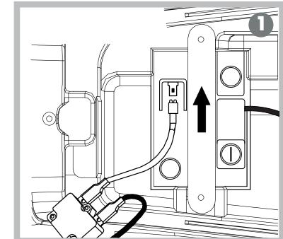
1. Unscrew and open the seat. Connect battery with **RED** wire. Then screw the seat back in place.
