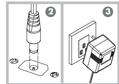
2. Plug into the jack. Connector jack is located at the back of the Trike body.
